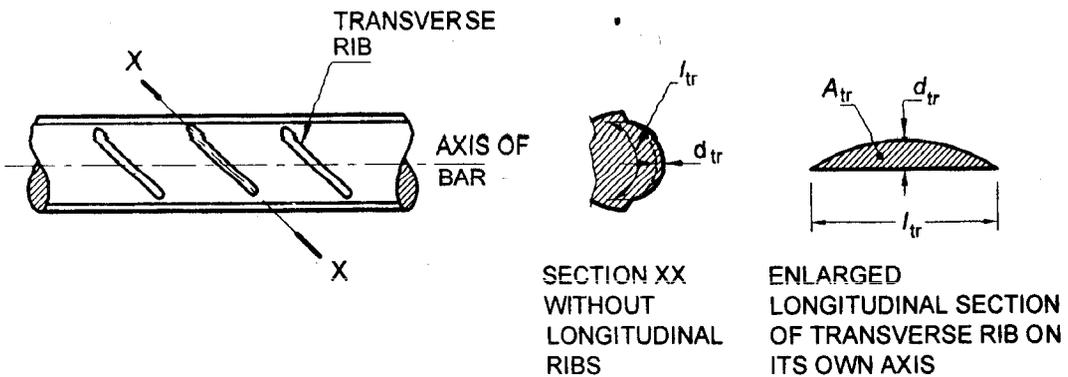
NOTE— $A_{tr}$ ,  $d_{tr}$  and  $l_{tr}$  represent longitudinal sectional area, height and length respectively of transverse rib
