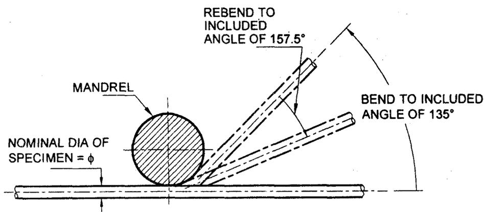
NOTE— $\phi$  Represents the nominal size in mm of the test piece.
